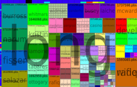
Treemap of PBS jobs from earlier output grouped by queue, user, and job id, colored by user, and sized by # of cpus (env repeat=15 grep -v '^fD' qstat -r | tree --color=f2 --fields=f3,f2,f1,f5)
