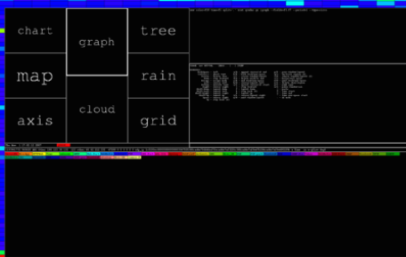
Savors console with top left showing 8 views arranged in 3-2-3 layout and details of current paused data line, top right showing graph view command and help, and bottom showing color legend
